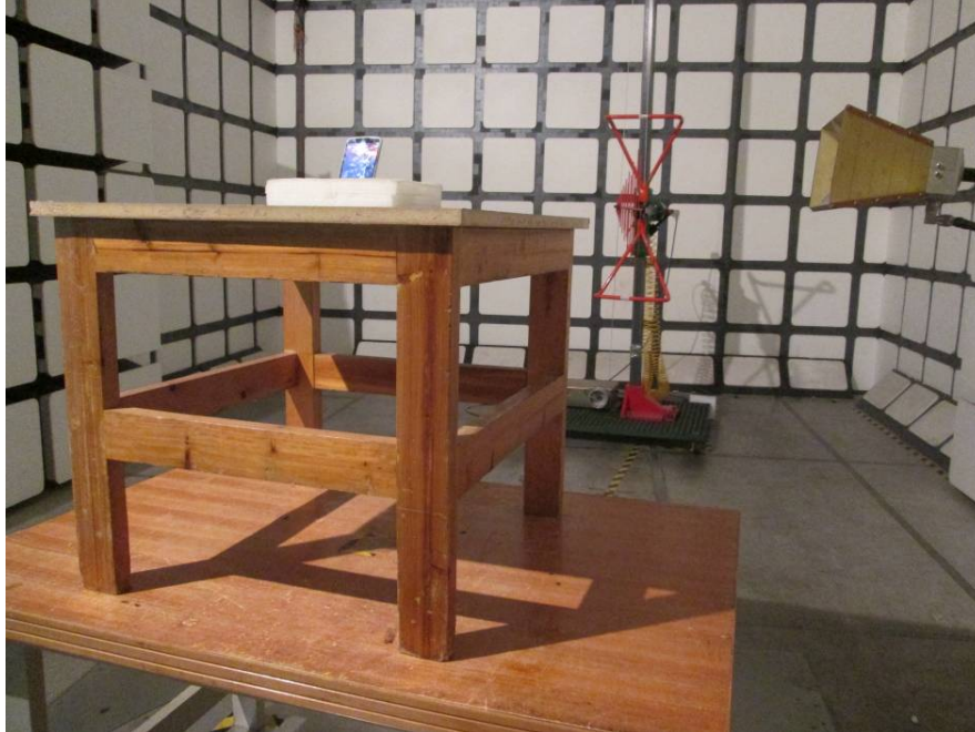
Radiated Emissions Test View (Below 1 GHz)
