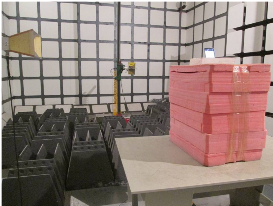
Radiated Emissions Test View (Above 1 GHz)
