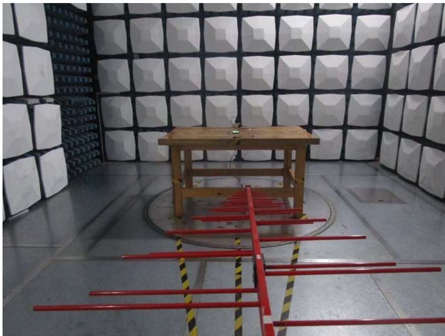
Radiated Emission Below 1GHz View
