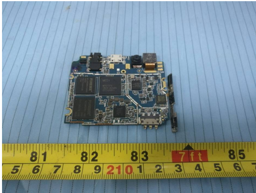
EUT – Main Board Bottom Shielding off View
