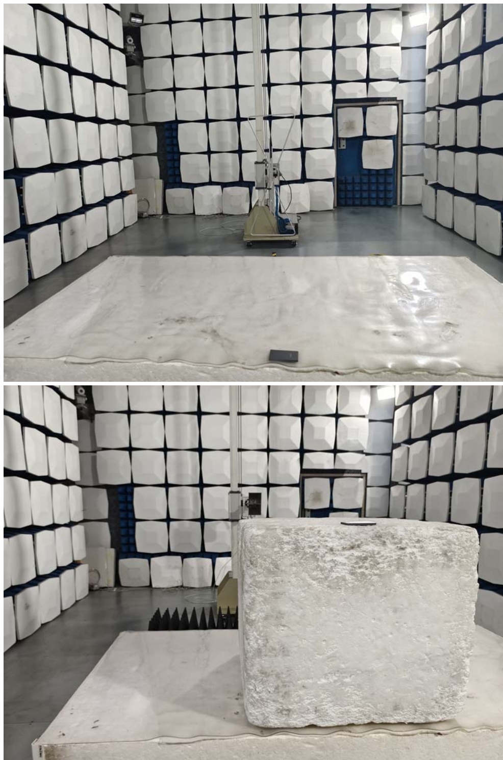
Radiated emission test view
