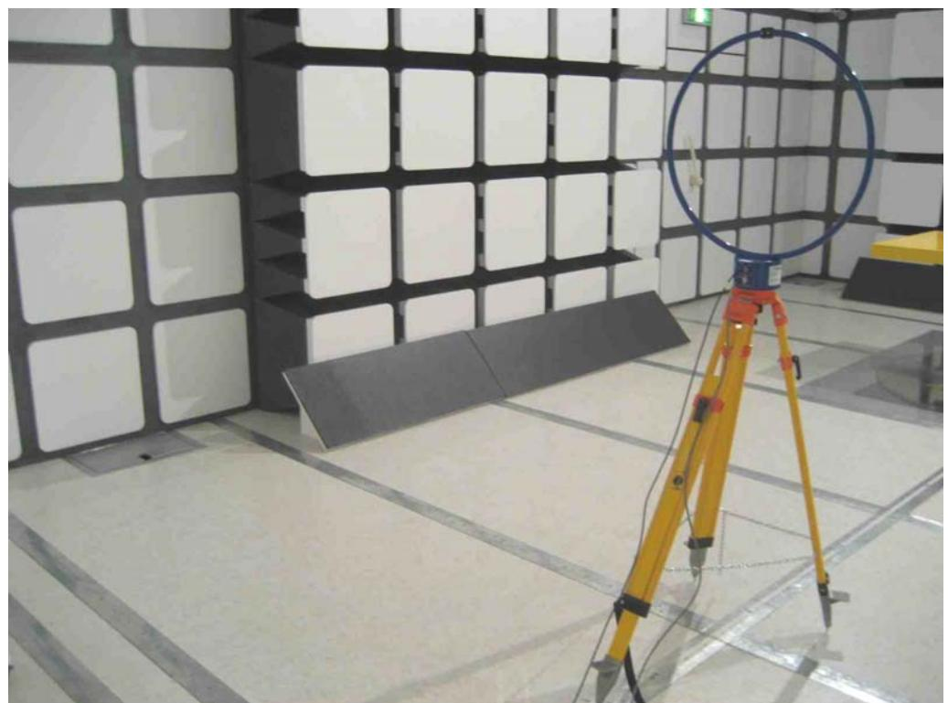
**Test Configuration: 30MHz~1GHz**
