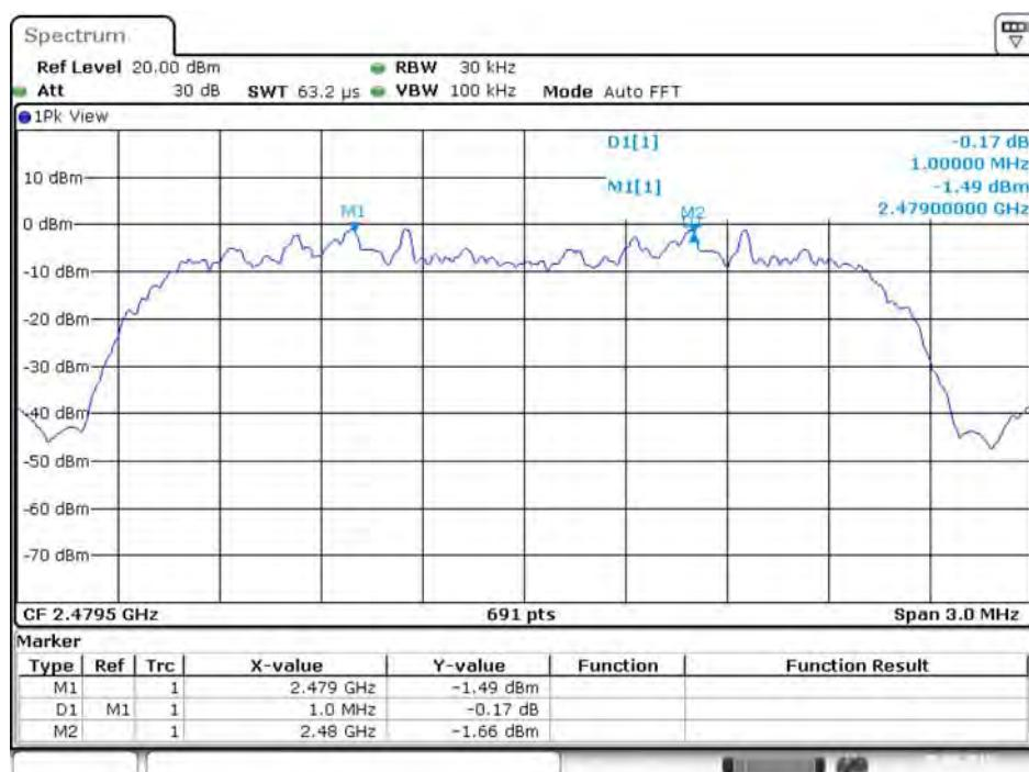
**20 dB Bandwidth Plot on EDR (8DPSK) 3 Mbps / Channel 0 / 2402 MHz**
