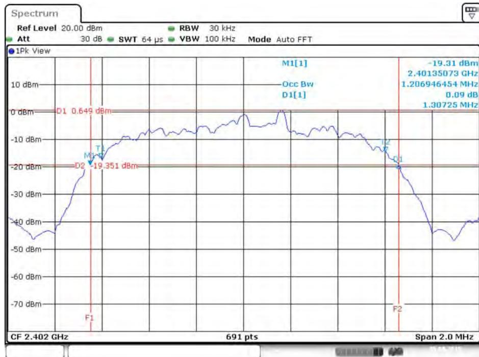
**20 dB Bandwidth Plot on EDR (8DPSK) 3 Mbps / Channel 39 / 2441 MHz**
