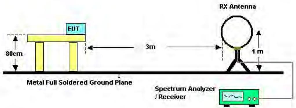
For Radiated Emissions: 30MHz~1GHz
