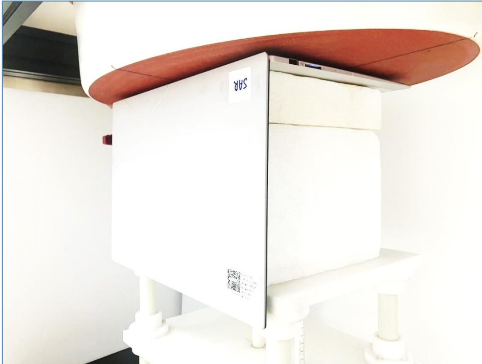
Setup for SAR Testing (Body, Bottom Surface of Base at 0 mm)
