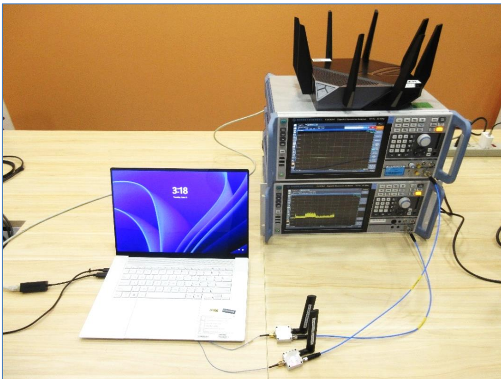
Setup for Conducted Power Testing (Test Scenario 2 and 5)
