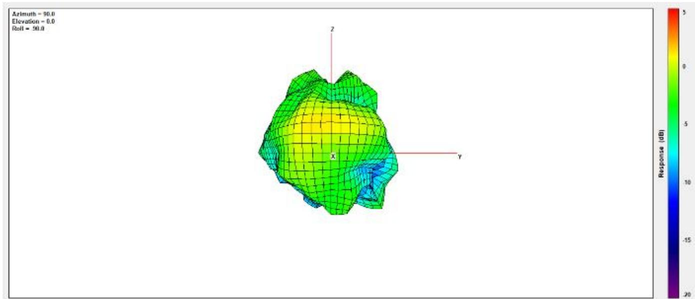
Max Antenna 3D Radiation Pattern 5150-5250 MHz
