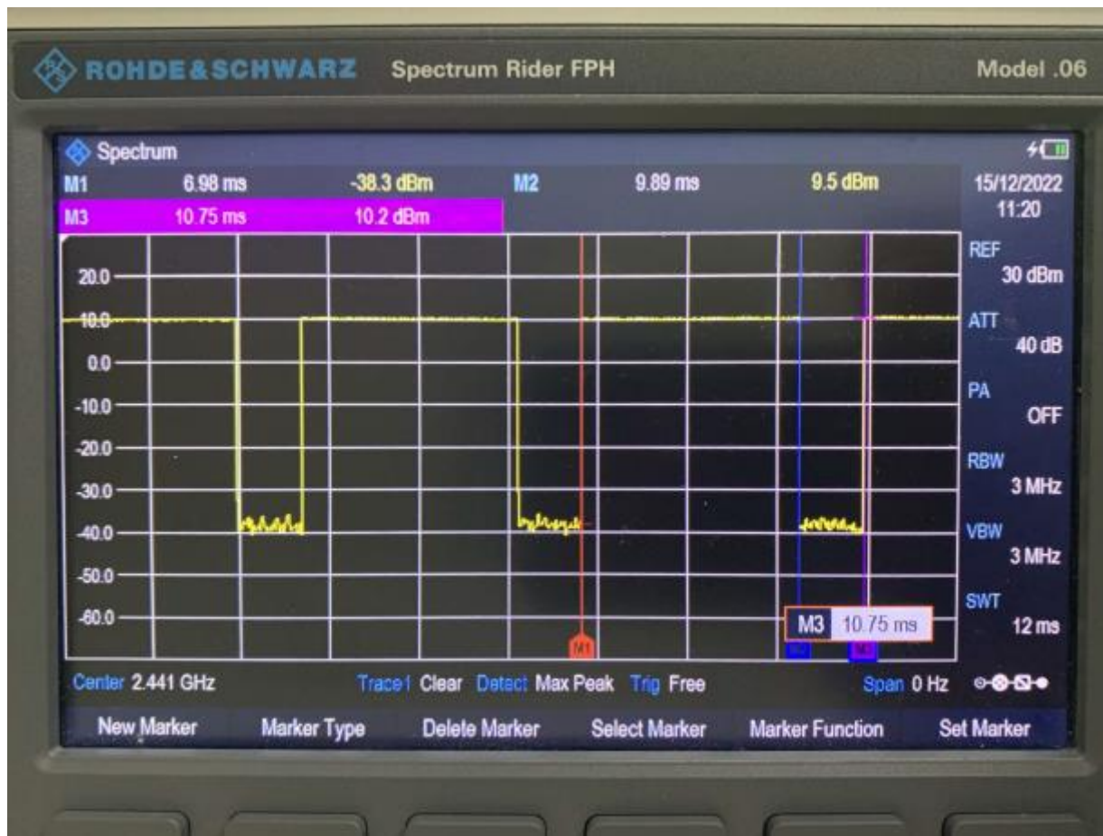
Time-domain plot for Bluetooth transmission signal
