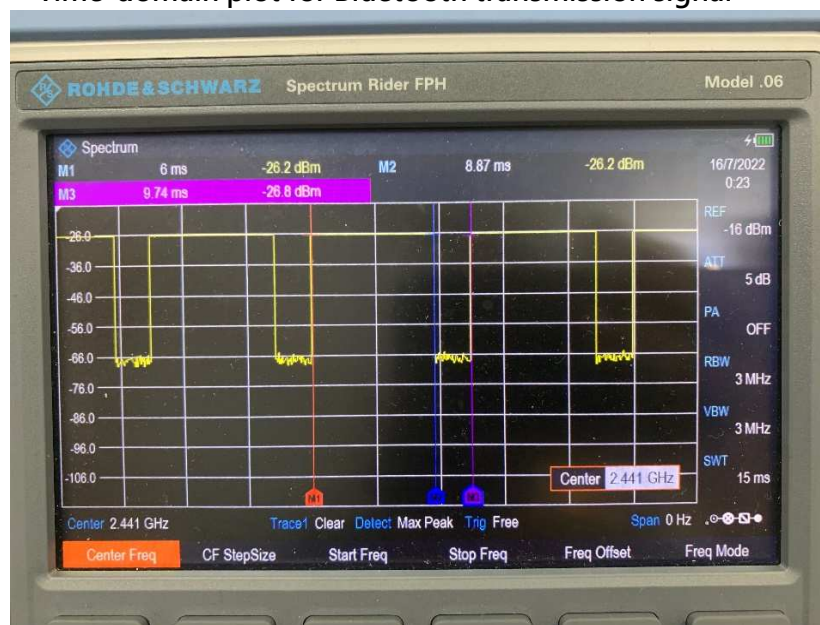
Time-domain plot for Bluetooth transmission signal
