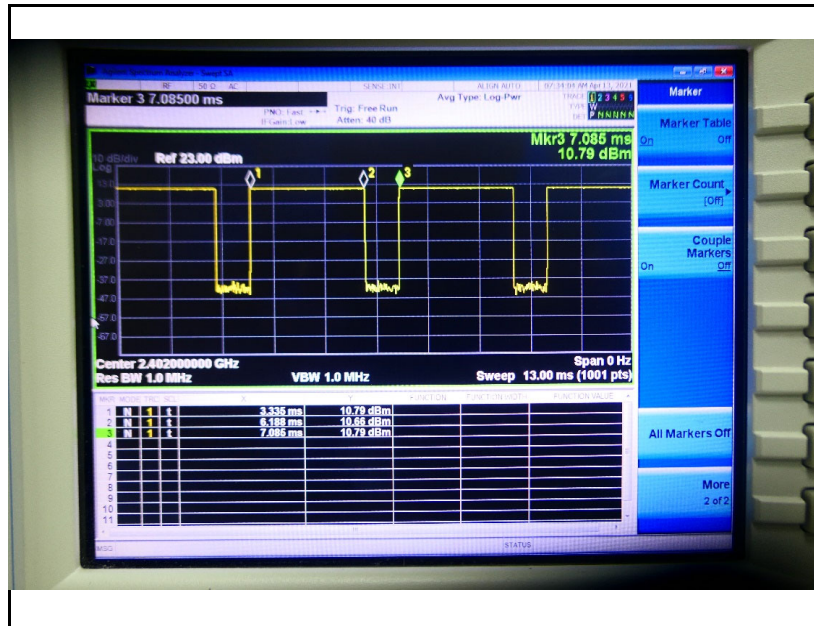
Time-domain plot for Bluetooth transmission signal
