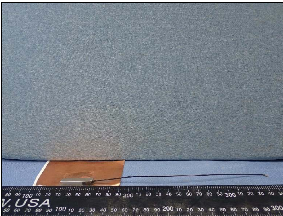
PIFA Antenna (Model: RFMTA340718EMLB302)
