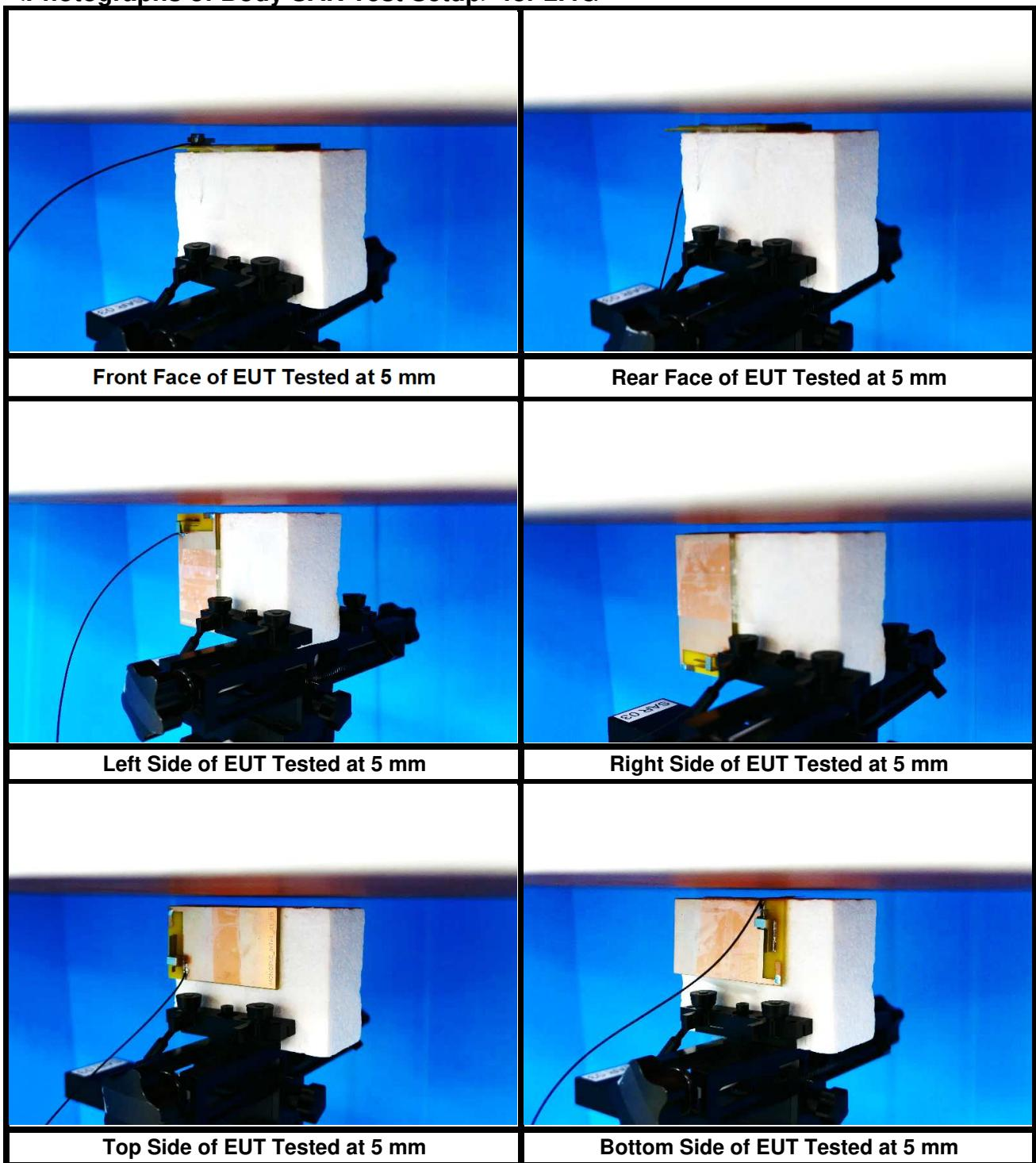
**<Photographs of Body SAR Test Setup> for 5G/6G**
