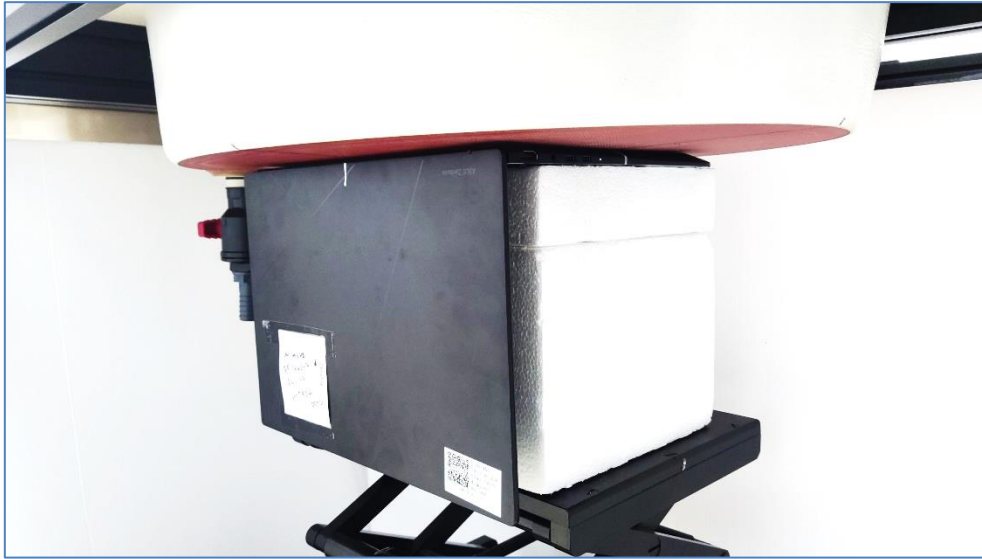
Setup for SAR Testing (Body, Bottom Surface at 0 mm)
