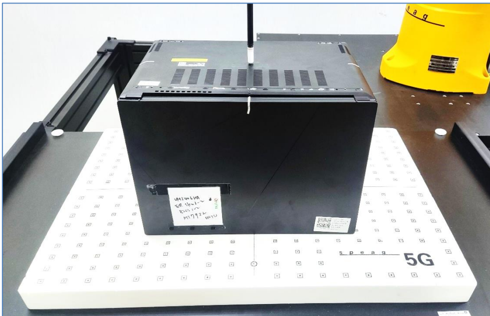
Setup for Power Density Testing (Bottom Surface at 2 mm)
