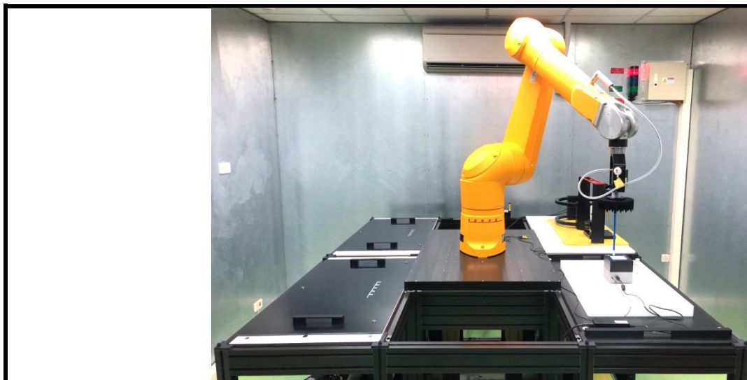
Fig-3.2 SPEAG DASY6 System
