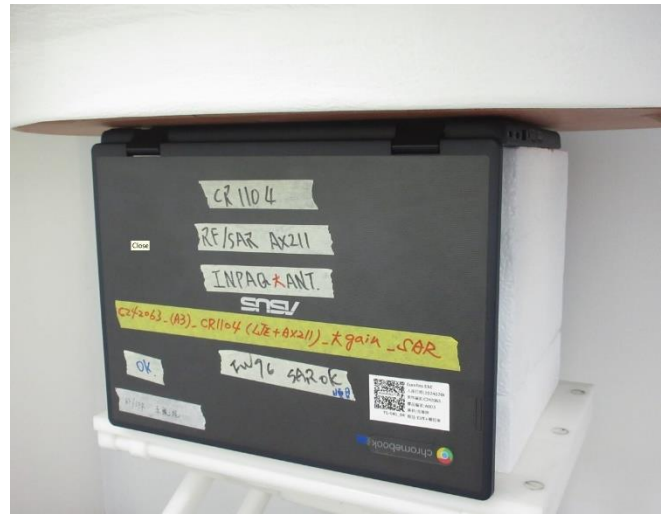
Testing Setup for Body, Bottom of Laptop at 0 mm
