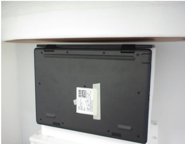
Testing Setup for Body, Back of Display Screen at 25 mm
