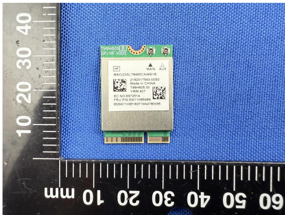
RF MODULE TOP VIEW -MT7920 (WITH SHIELDING)
