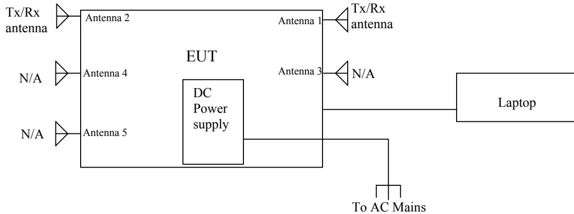
5 GHz Single band antenna setup:
