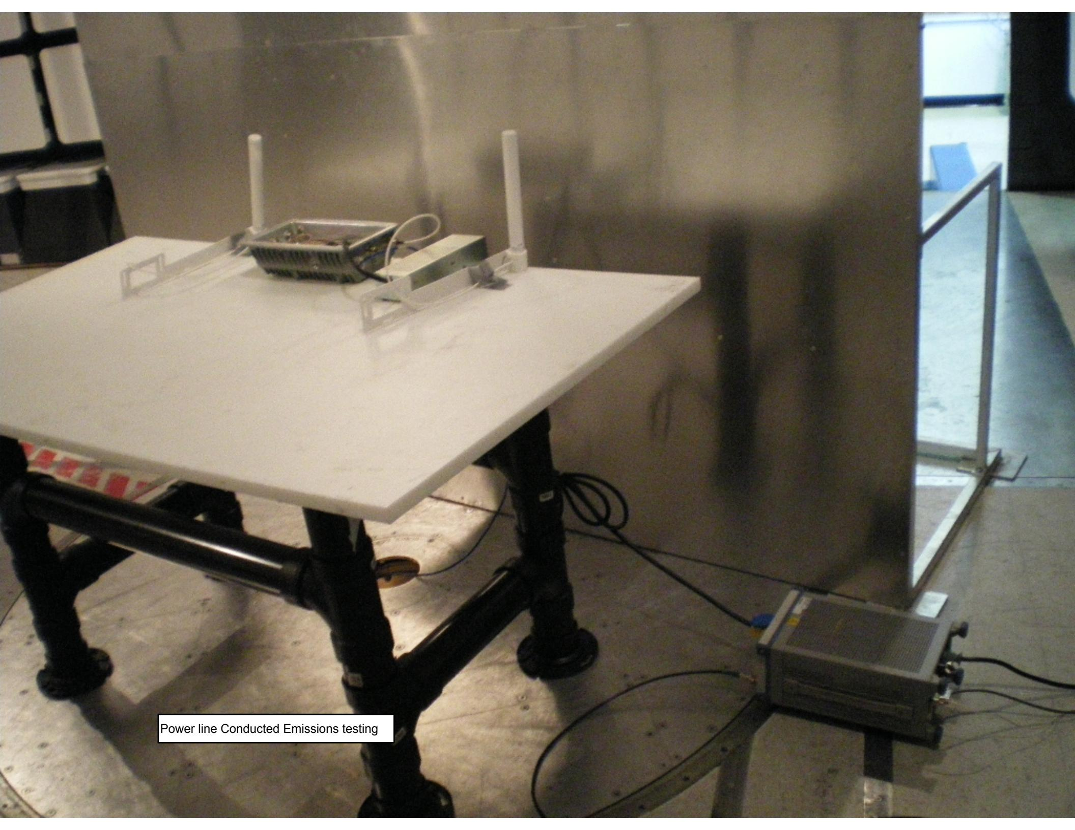
Power line Conducted Emissions testing
