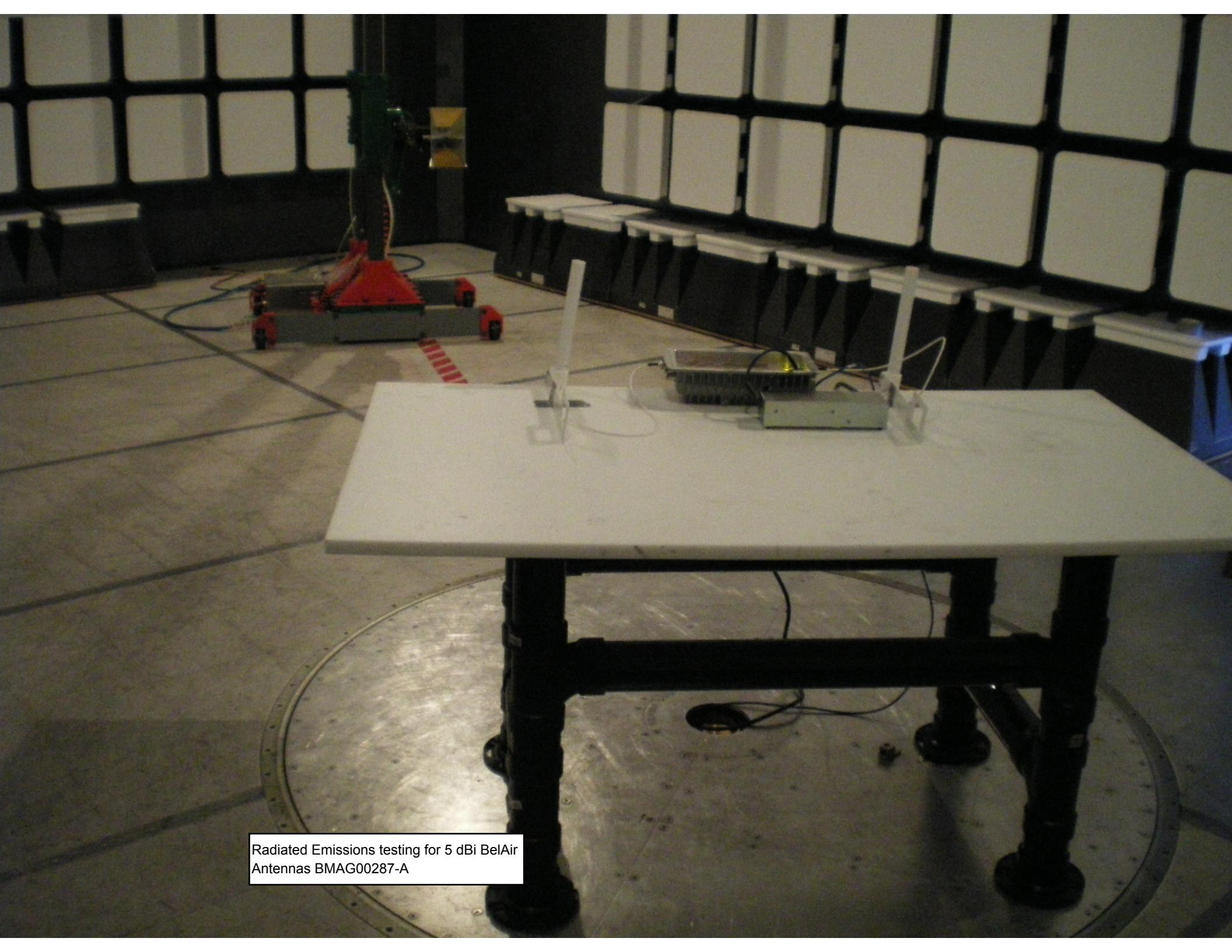
Radiated Emissions testing for 5 dBi BelAir
