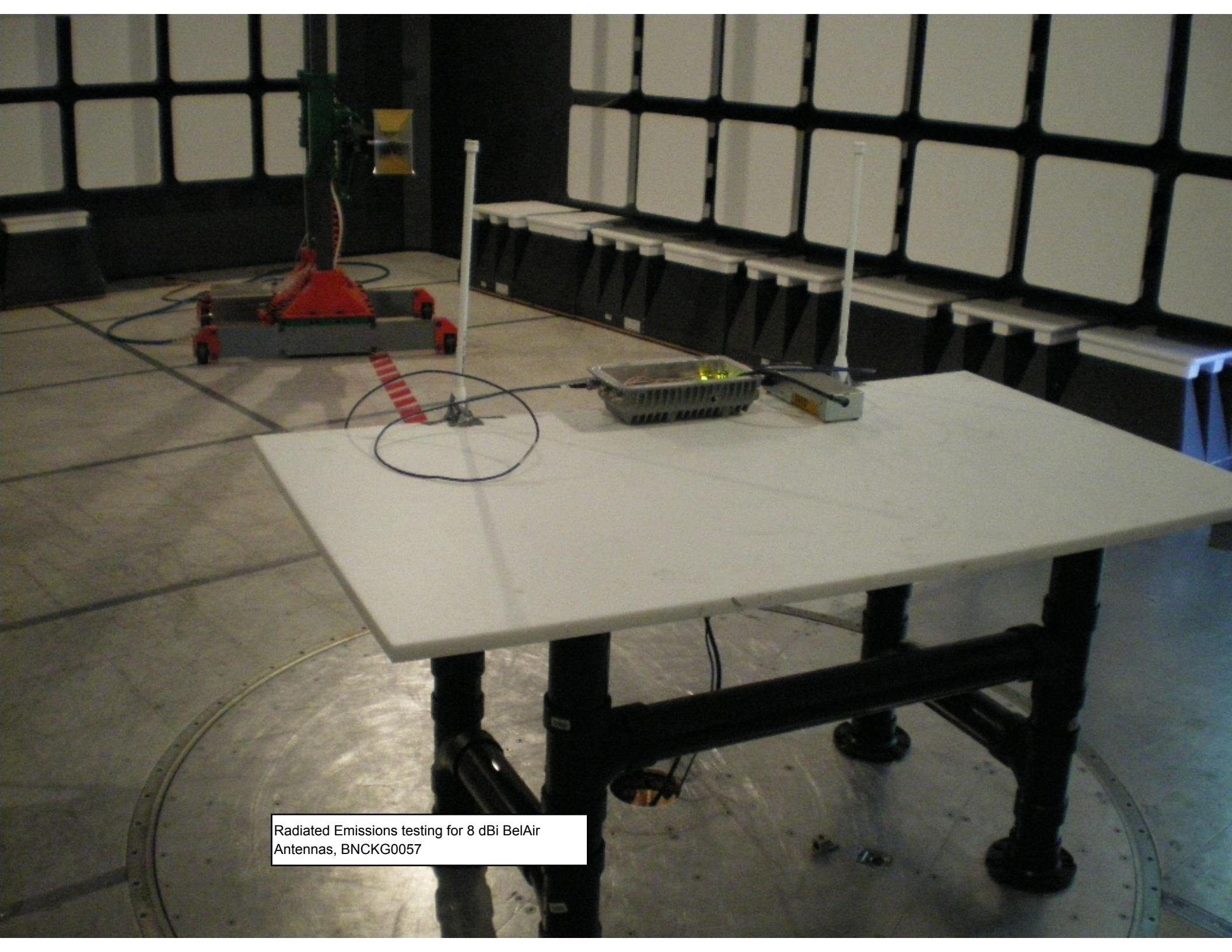
Radiated Emissions testing for 8 dBi BelAir
