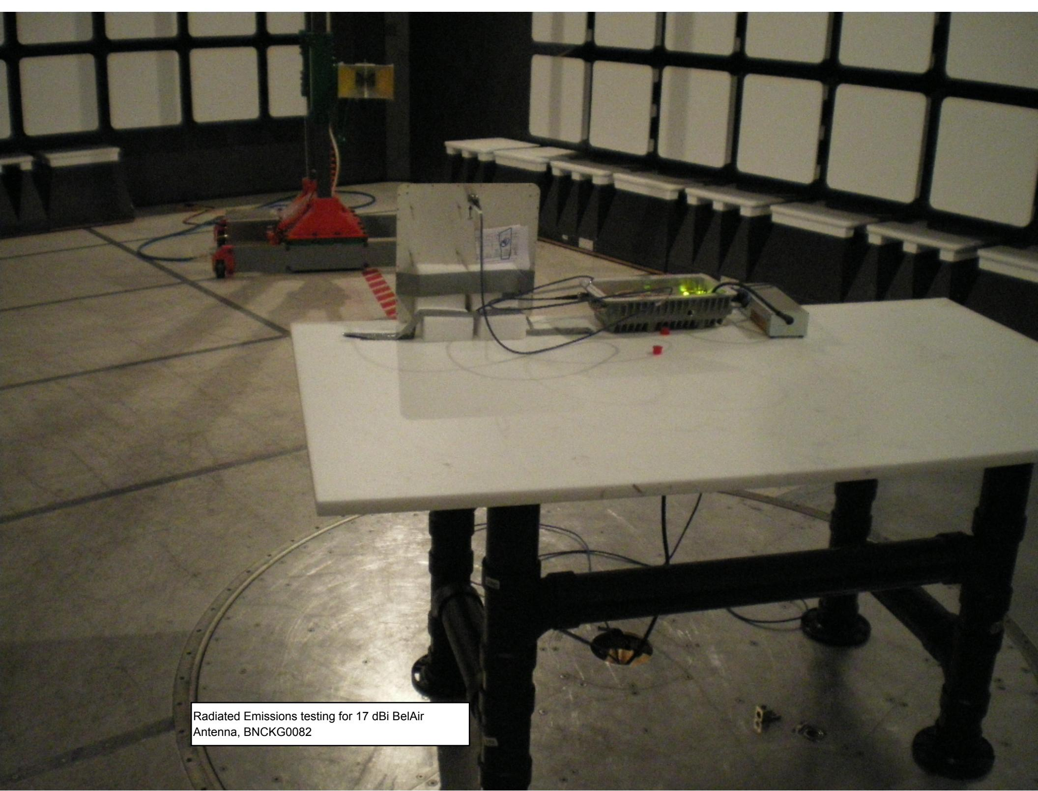
Radiated Emissions testing for 17 dBi BelAir
