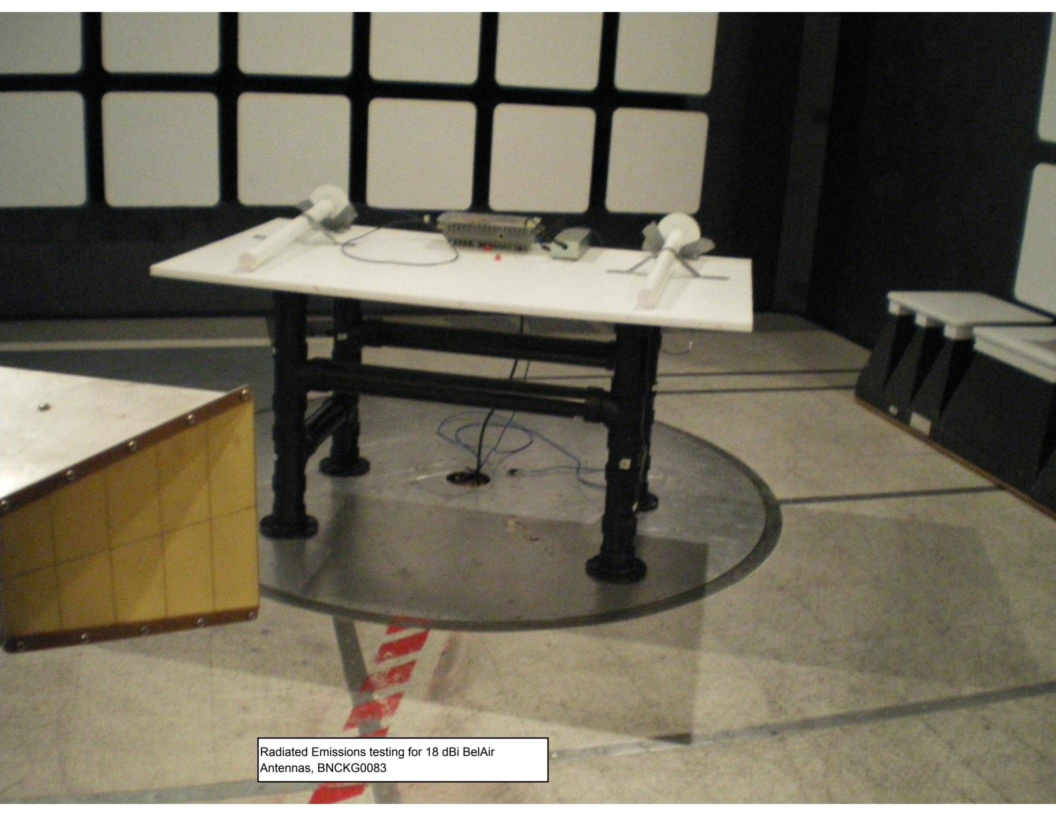
Radiated Emissions testing for 18 dBi BelAir
