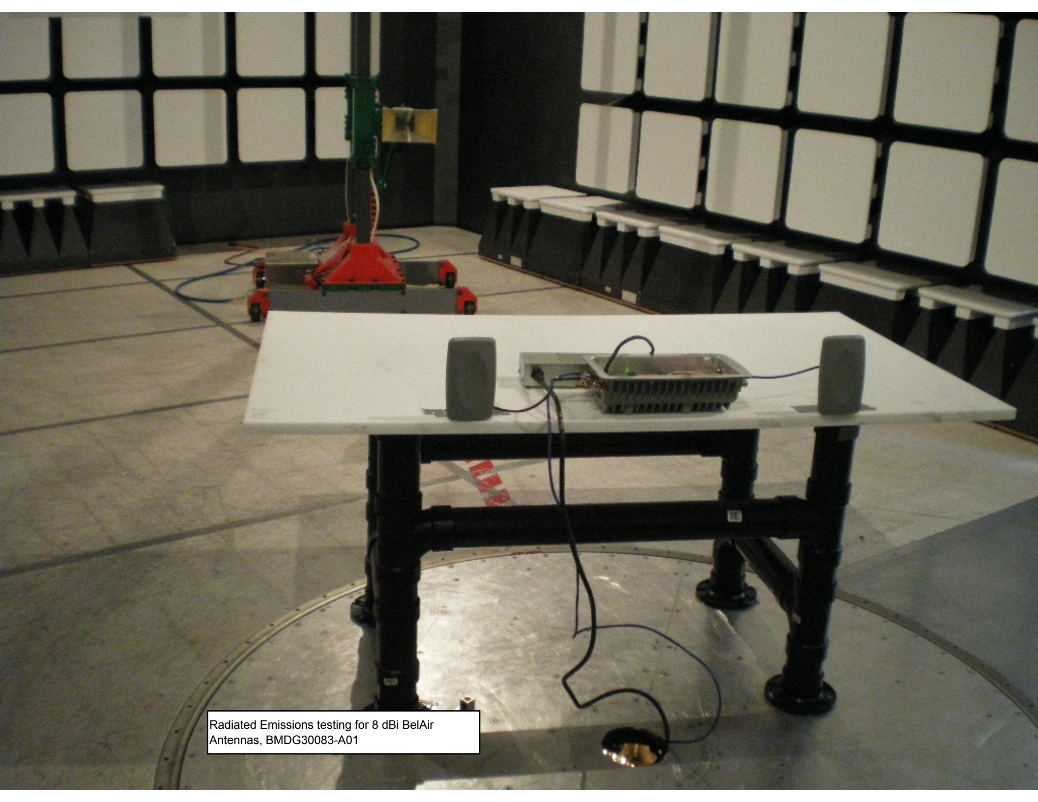
Radiated Emissions testing for 8 dBi BelAir
