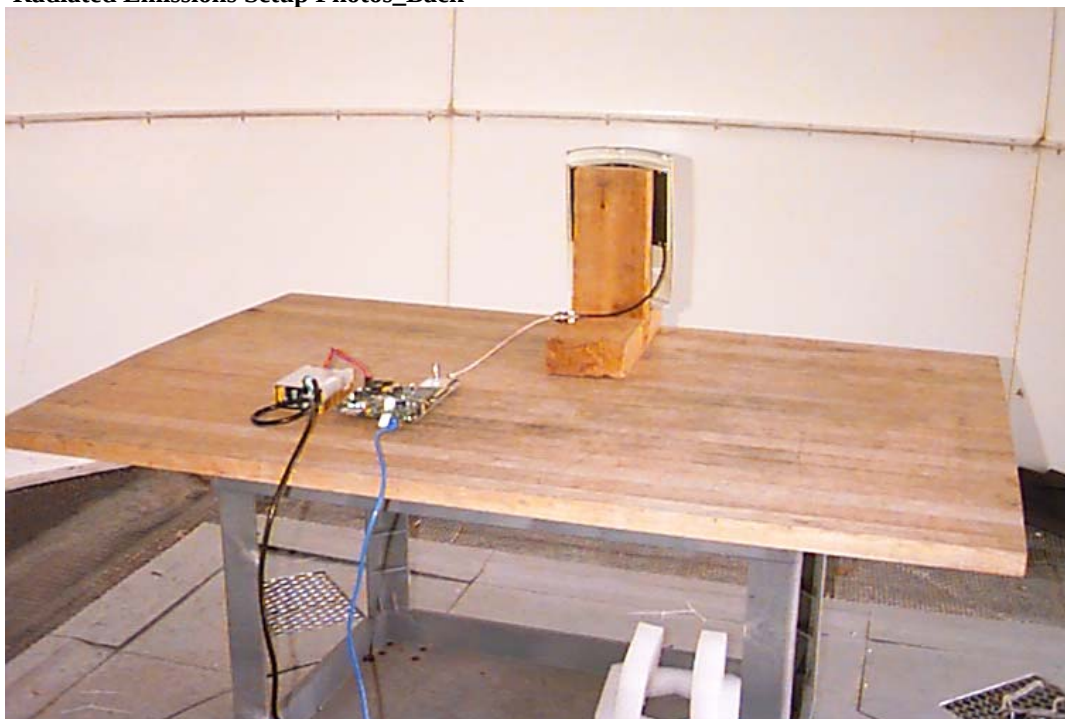
Radiated Emissions Setup Photos_Back
