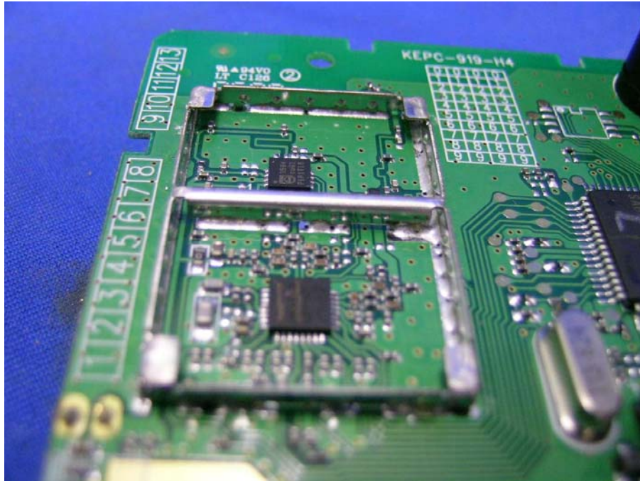
Base Unit Oscillator PCB comp side (View 3)
