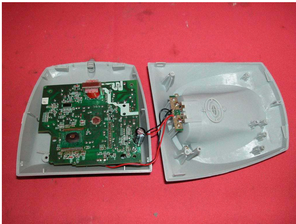
Base Main PCB comp side (View 1)
