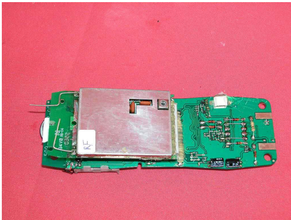
Handset Main PCB comp side (View 1)
