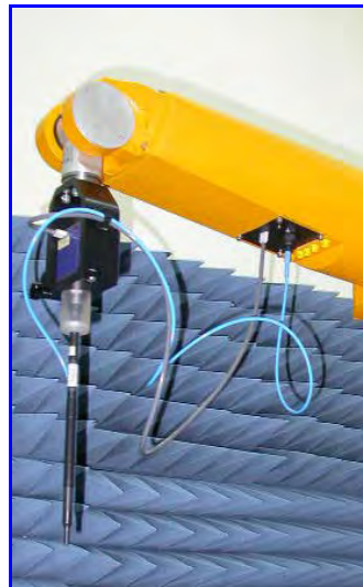
Figure 3. Probe setup on robot
