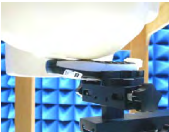
Figure 14. Right Head SAR Test Setup (Cheek)
