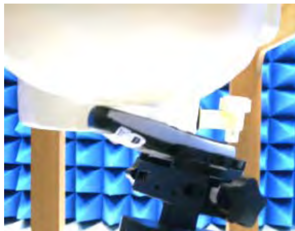
Figure 15. Right Head SAR Test Setup (Tilted)
