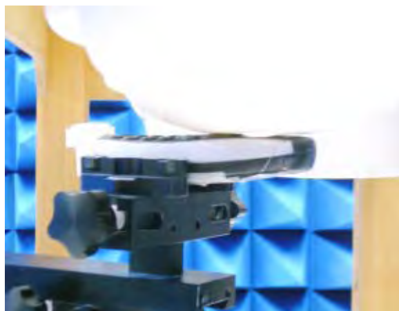
Figure 16. Left Head SAR Test Setup (Cheek)
