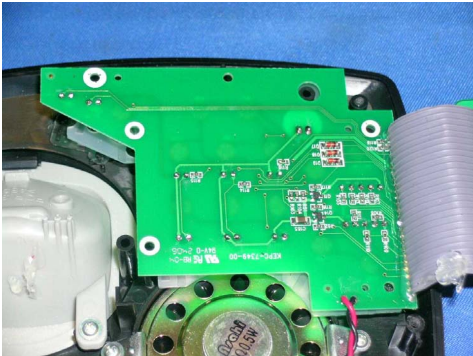
Base Unit another Main PCB solder side
