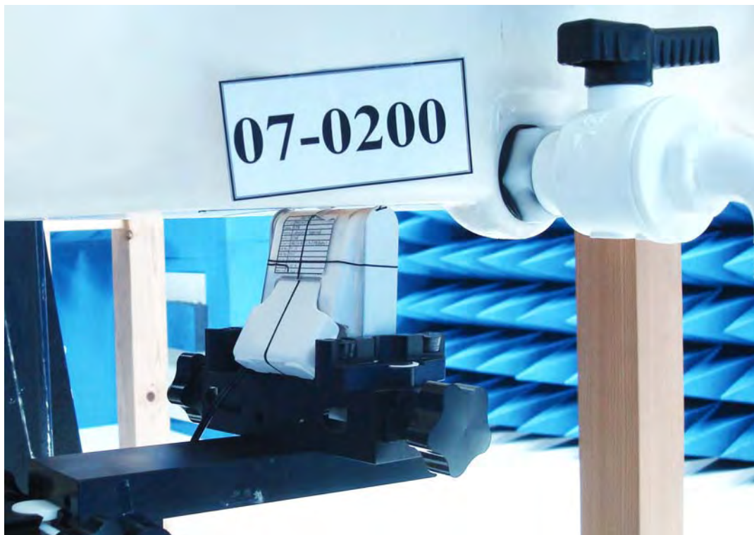
Figure 14. Body SAR Test Setup (Flat Section)
