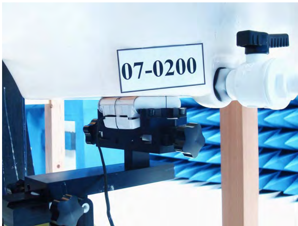
Figure 12. Body SAR Test Setup (Flat Section)
