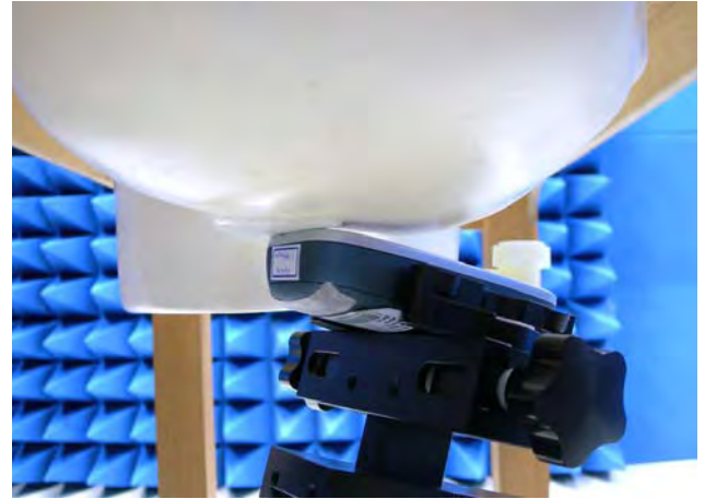
Figure 17.Right Head SAR Test Setup (Tilted)
