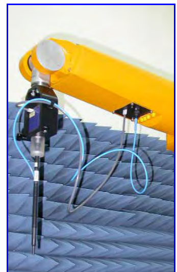
Figure 10. Probe setup on robot
