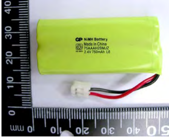
Figure 2. Battery (Ni-MH 2.4V , 750mAh)
