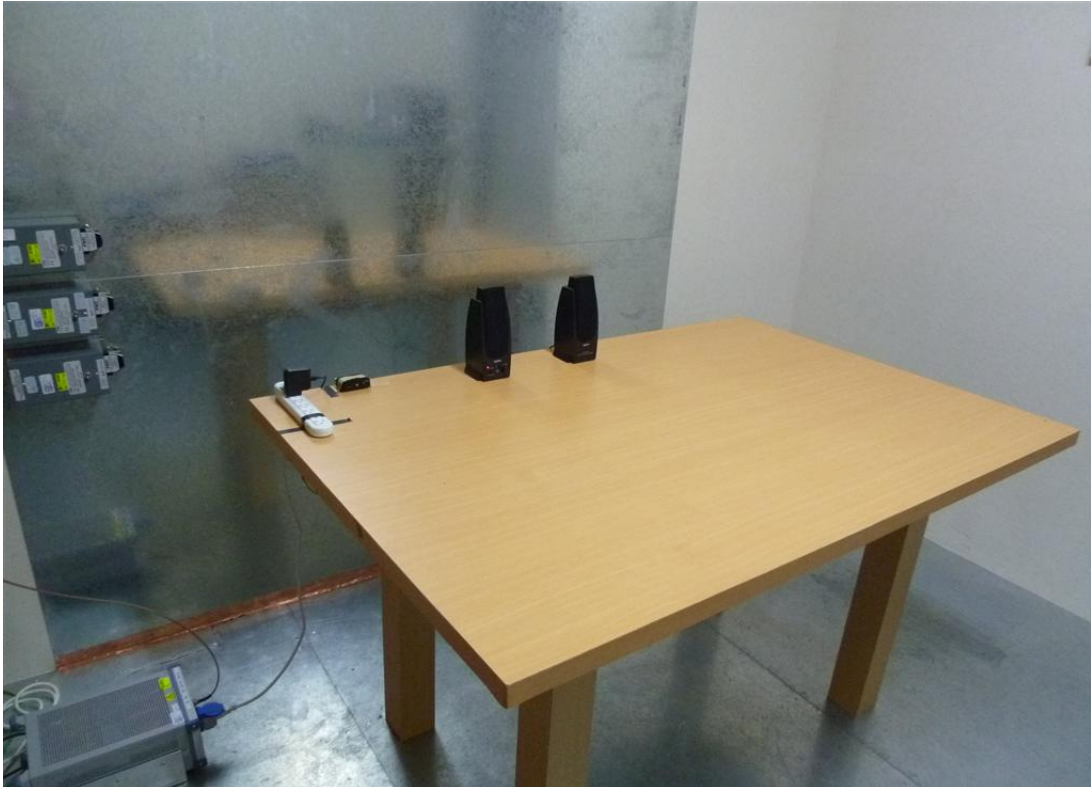
Photograph 5: Set-up for Mains Conducted testing, front view
