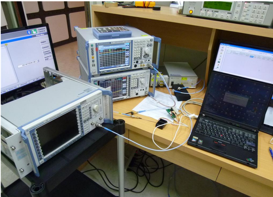
Photograph 4: Set-up for Conducted testing
