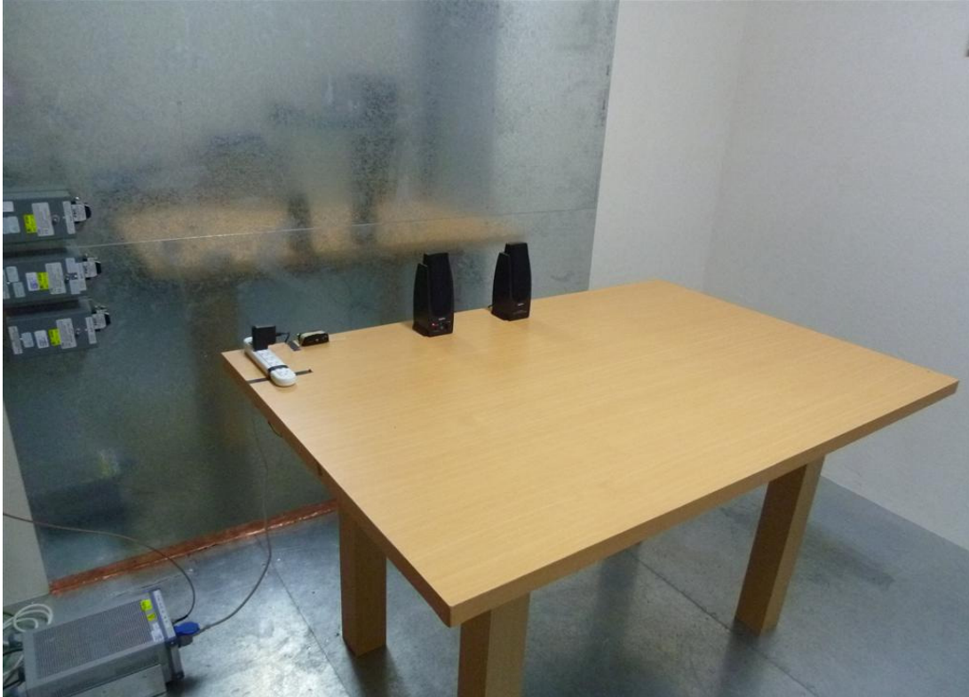
Photograph 5: Set-up for Mains Conducted testing, front view
