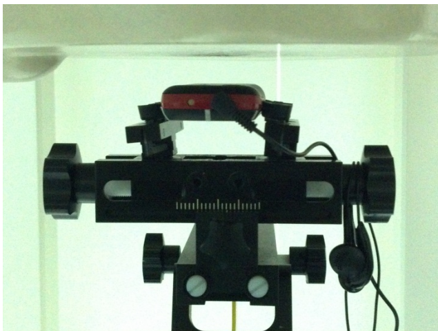
Back of the DUT with Phantom 1.5cm Gap (w/ headset)
