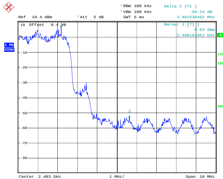
Fig.11. Frequency Band Edges: 8DPSK, Channel 78, Hopping Off
