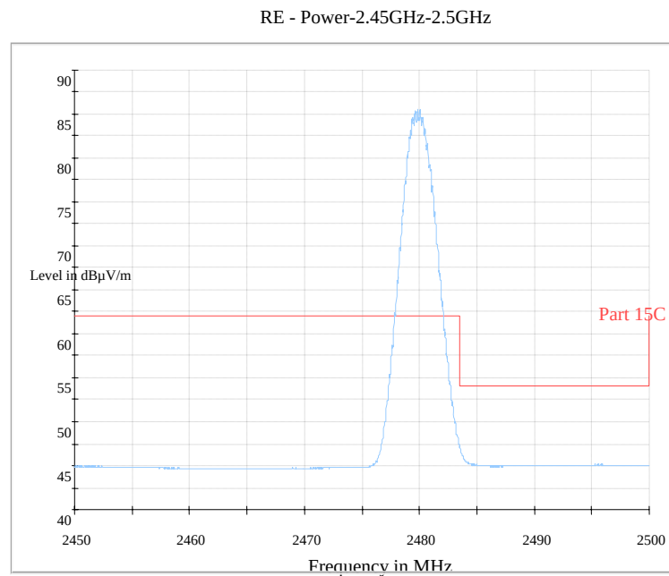
Fig.92. Radiated emission (Power): 8DPSK, high channel
