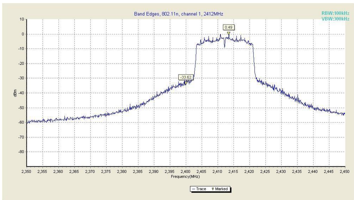
Fig. 23 Band Edges (802.11 n-20MHz, Ch 1)
