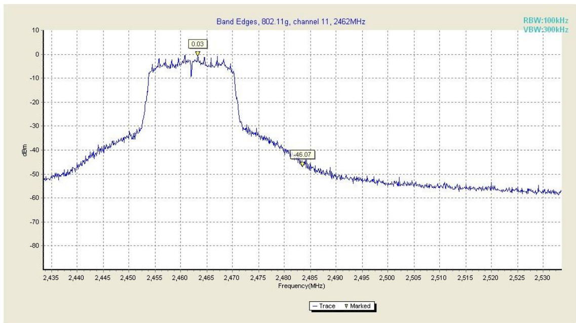
Fig. 22 Band Edges (802.11g, Ch 11)
