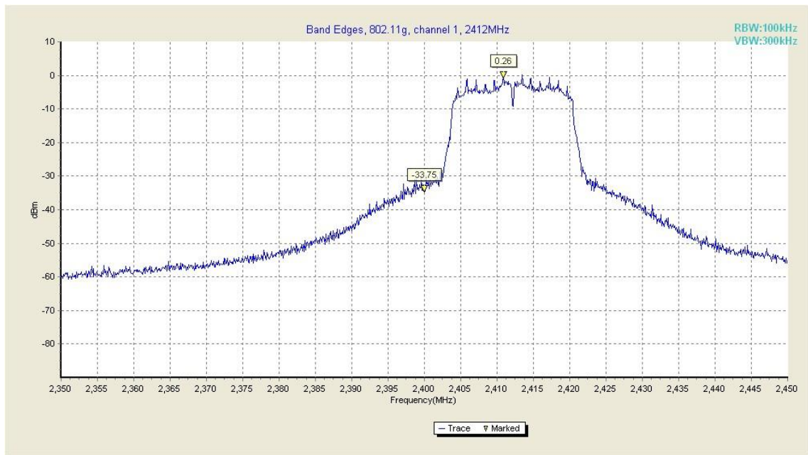
Fig. 21 Band Edges (802.11g, Ch 1)
