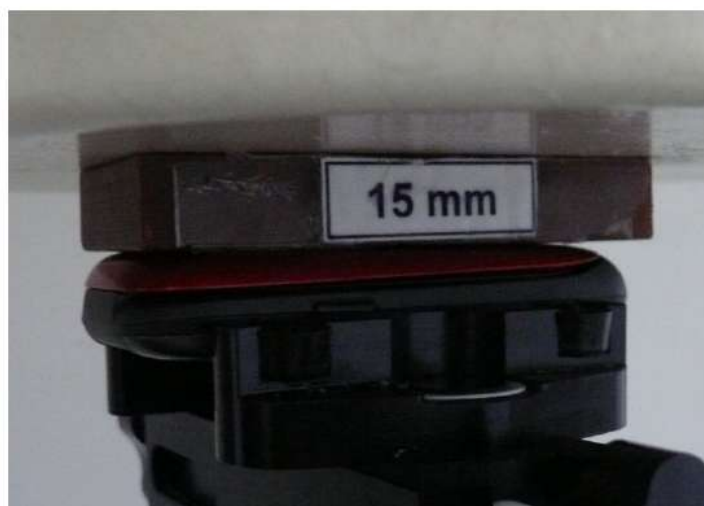
Picture 12: Body, The EUT display towards phantom, the distance from handset to the bottom of the Phantom is 15mm (The spacer was removed during testing, Close)
