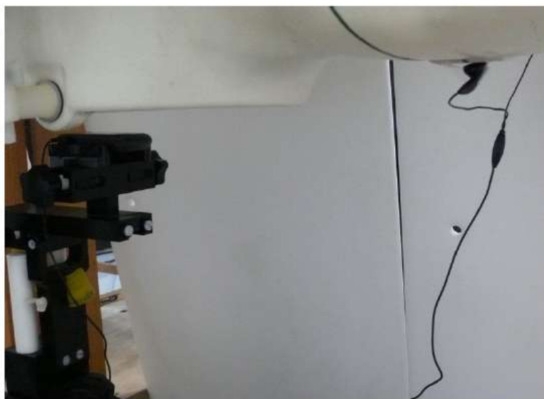
Picture 14: Body with earphone, The EUT display towards ground, the distance from handset to the bottom of the Phantom is 15mm (Close)
