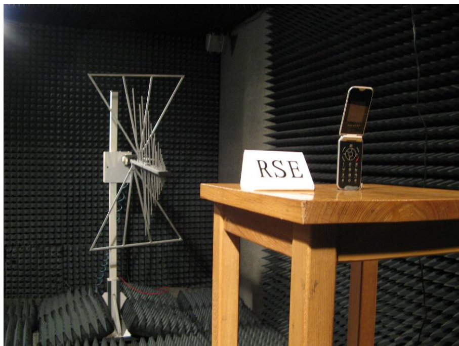
Pic C-2 Radiated Spurious Emission
