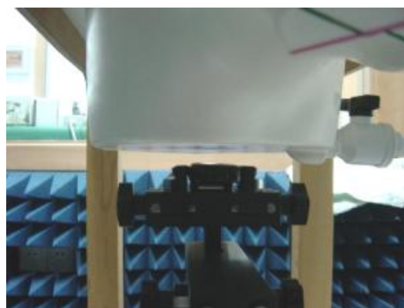
Fig.10 Photograph of the BodyWorn status
