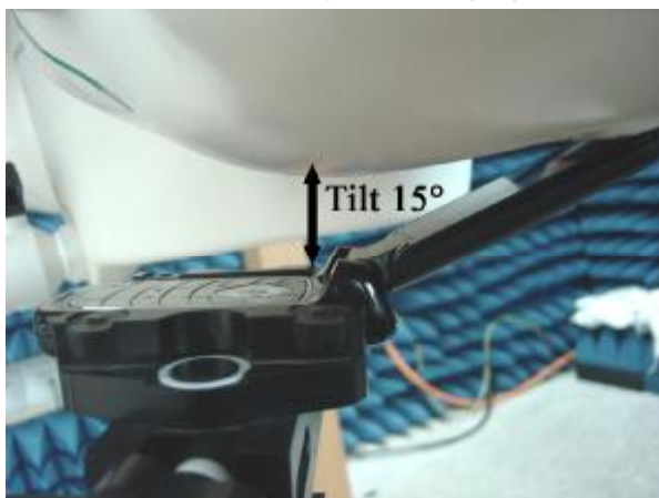
Fig.6 Photograph of the Left Hand Side Touch status
