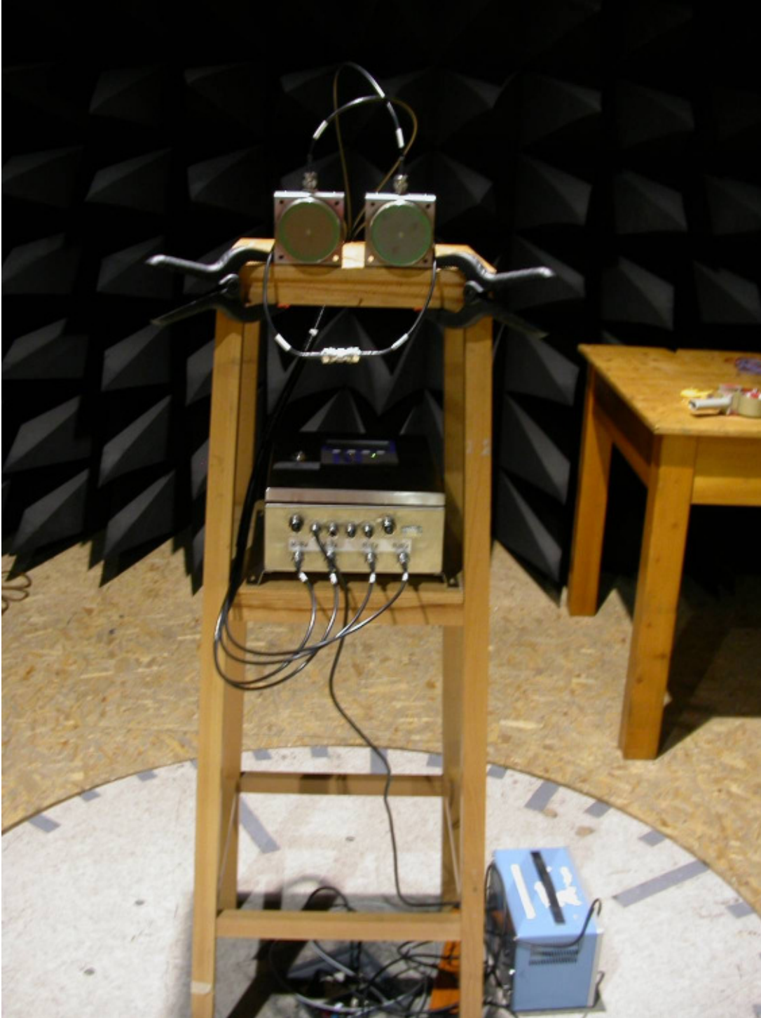
Spurious emissions measurement up to 12 GHz (Spiral antennas)
