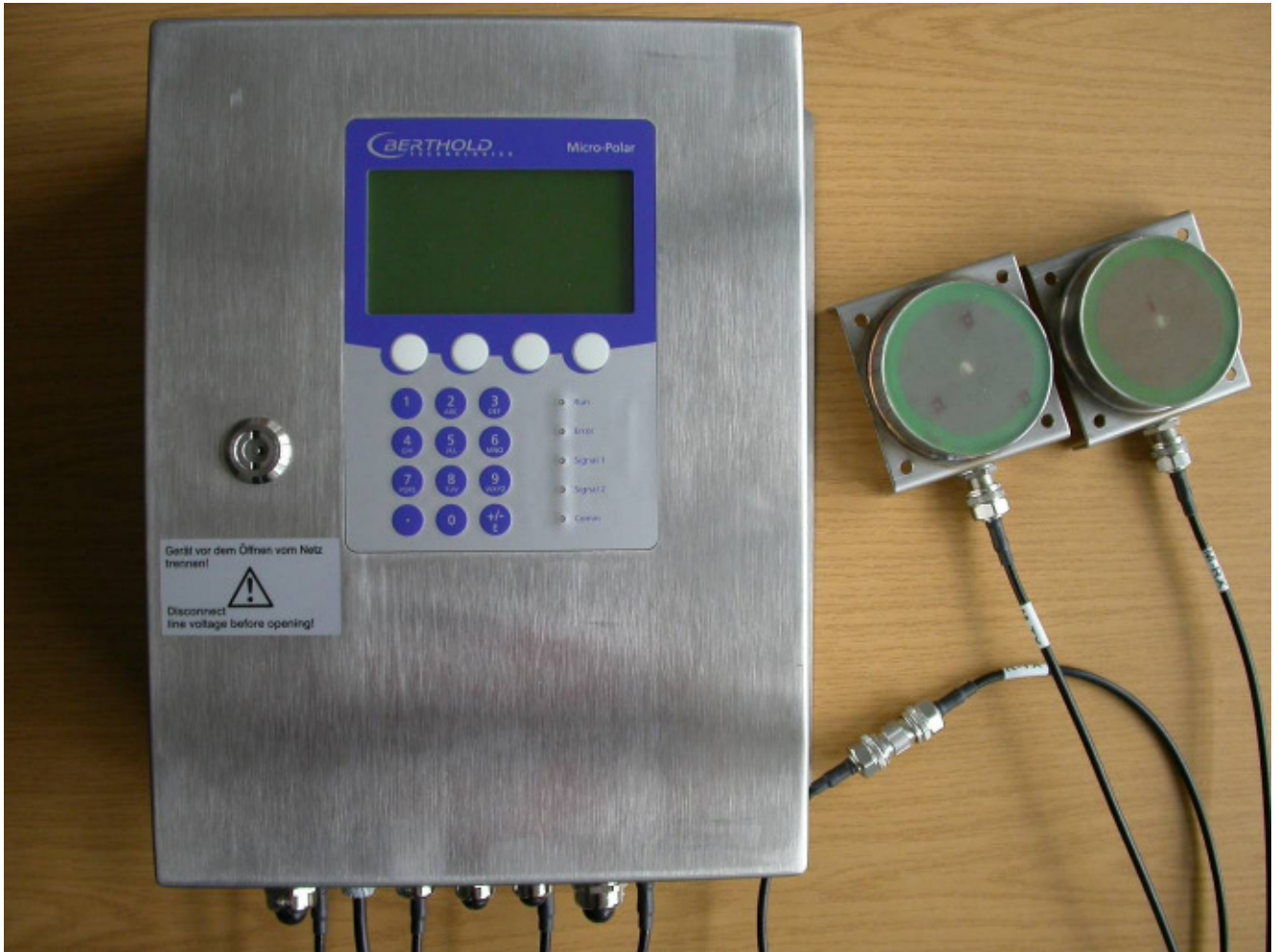
Front view of the EUT equipped with spiral antennas
