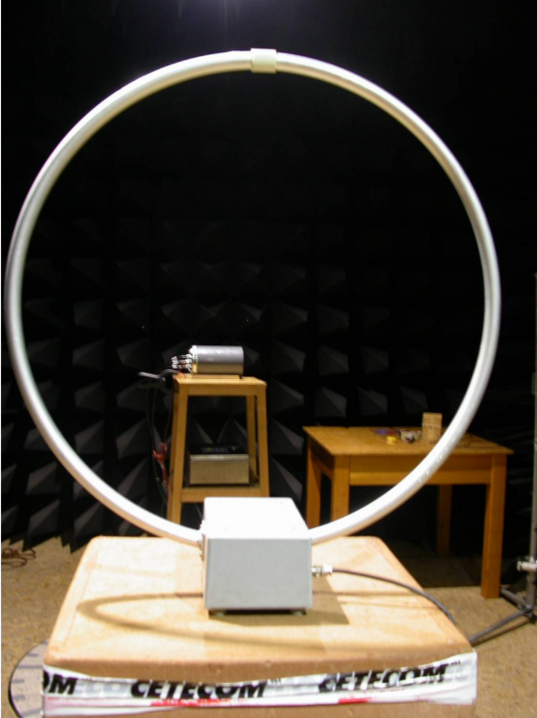
Spurious emissions measurement up to 30 MHz with a magnetic loop antenna
