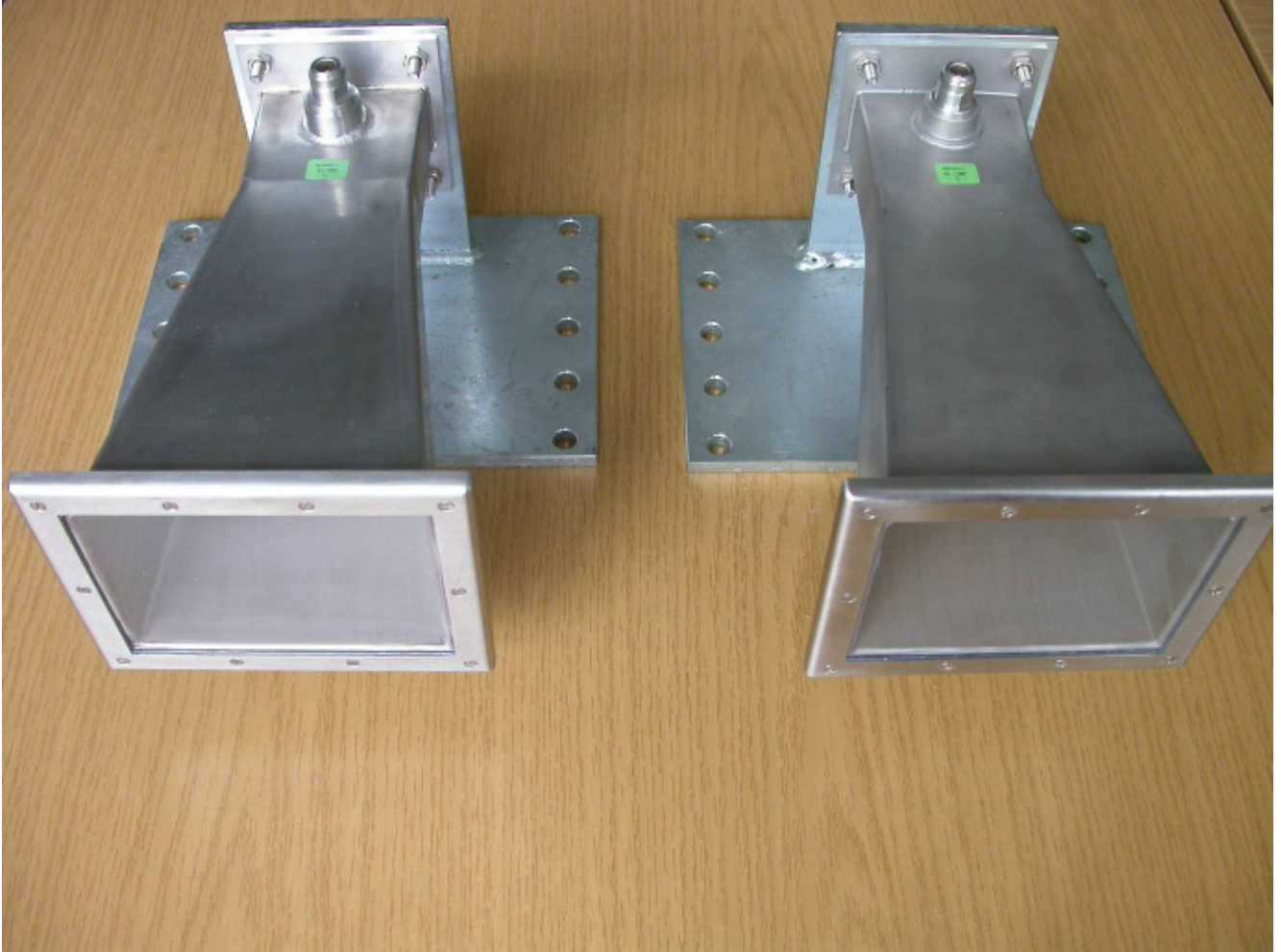
Tx and Rx Horn Antennas
