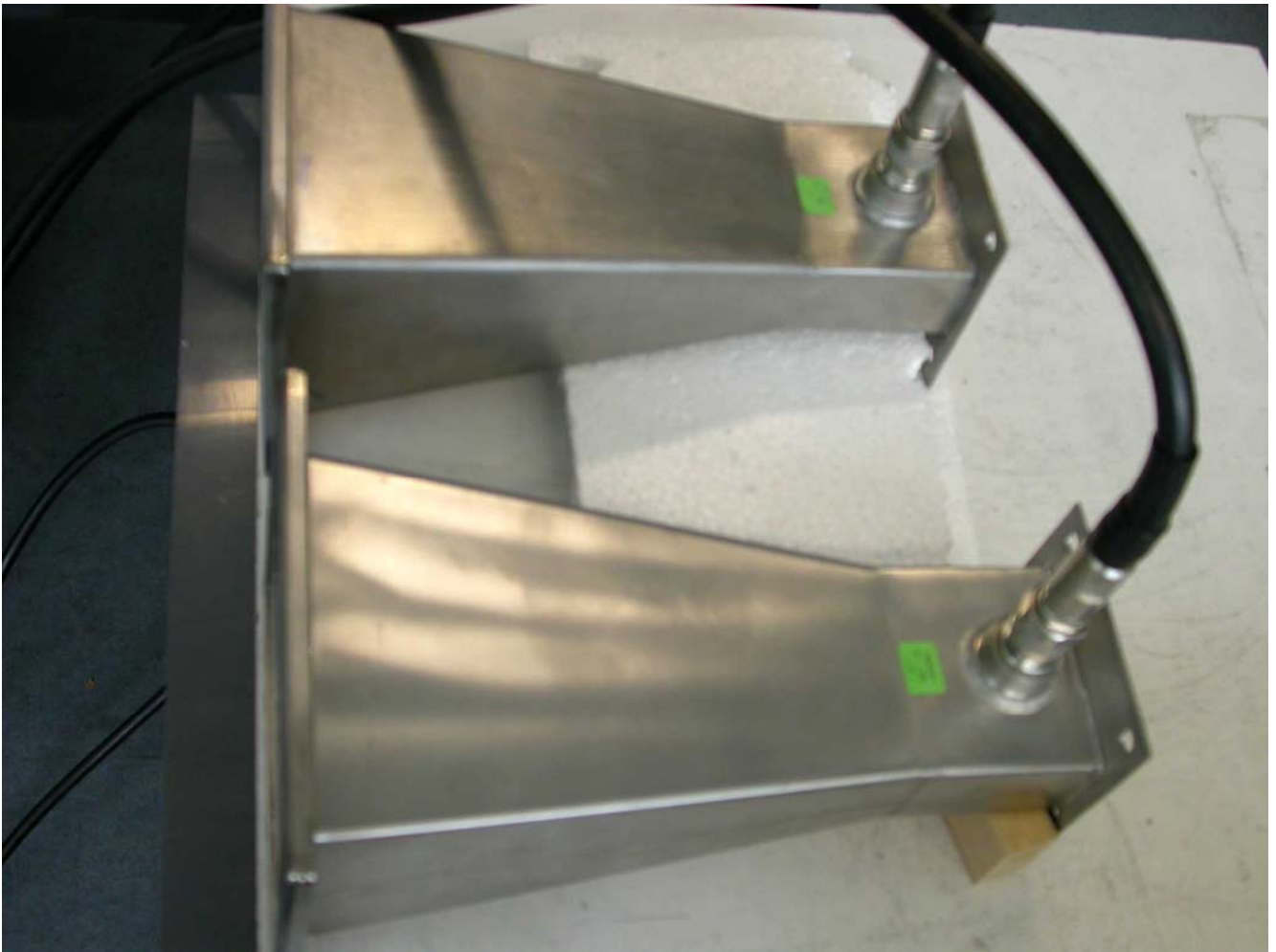
TX and RX horn antennas LB X60X-XX
