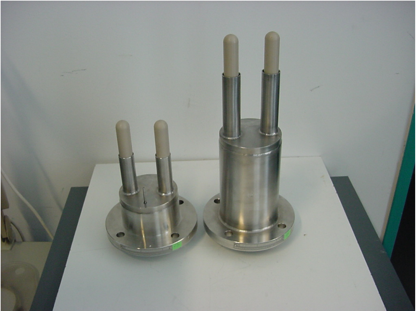
In tank sensor LB X650-XX (same antenna , different housings)
