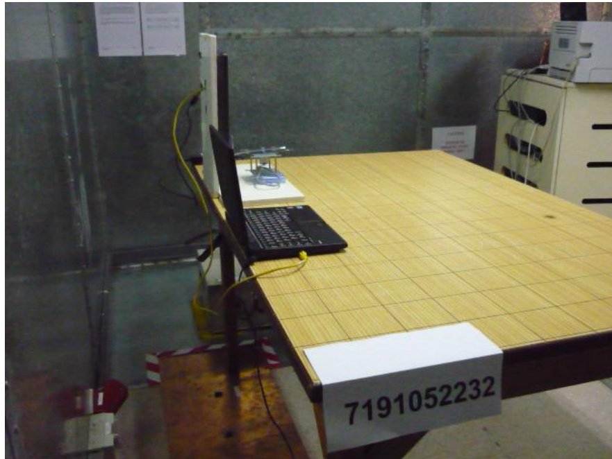
Conducted Emissions Test Setup (Rear View)
