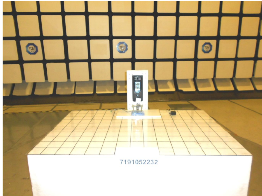
Radiated Emissions Test Setup (Front View)
