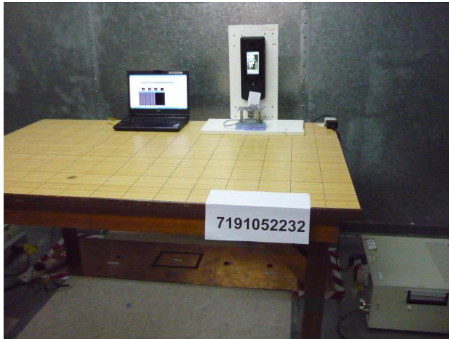
Conducted Emissions Test Setup (Front View)
