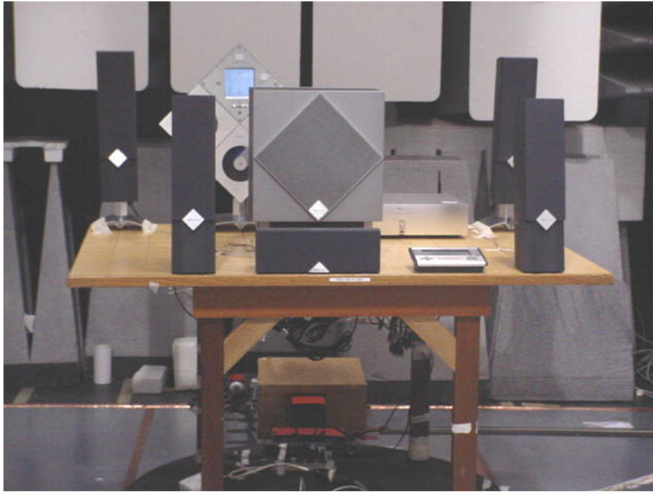
Radiated Emissions Setup (Front View)
