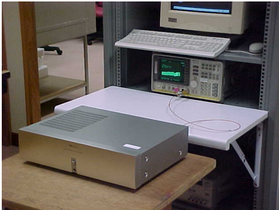
Carrier Frequency Separation Measurement Test Setup – AV Unit
