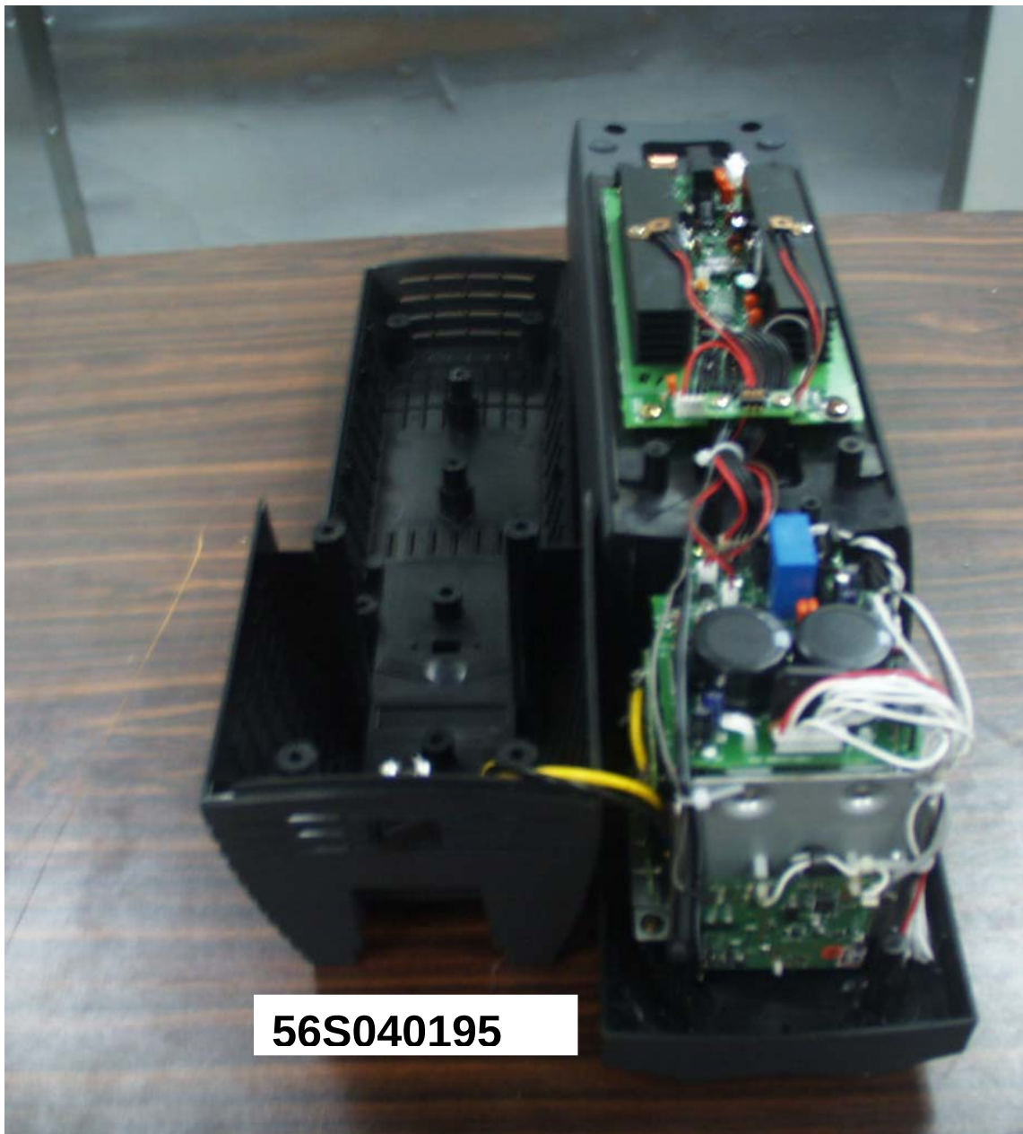
Rear Left/Right Speaker – Internal Layout
