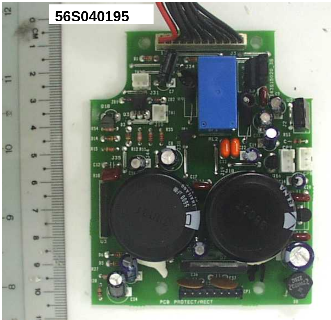
Rear Left/Right Speaker – Rectifier Board Component Side
