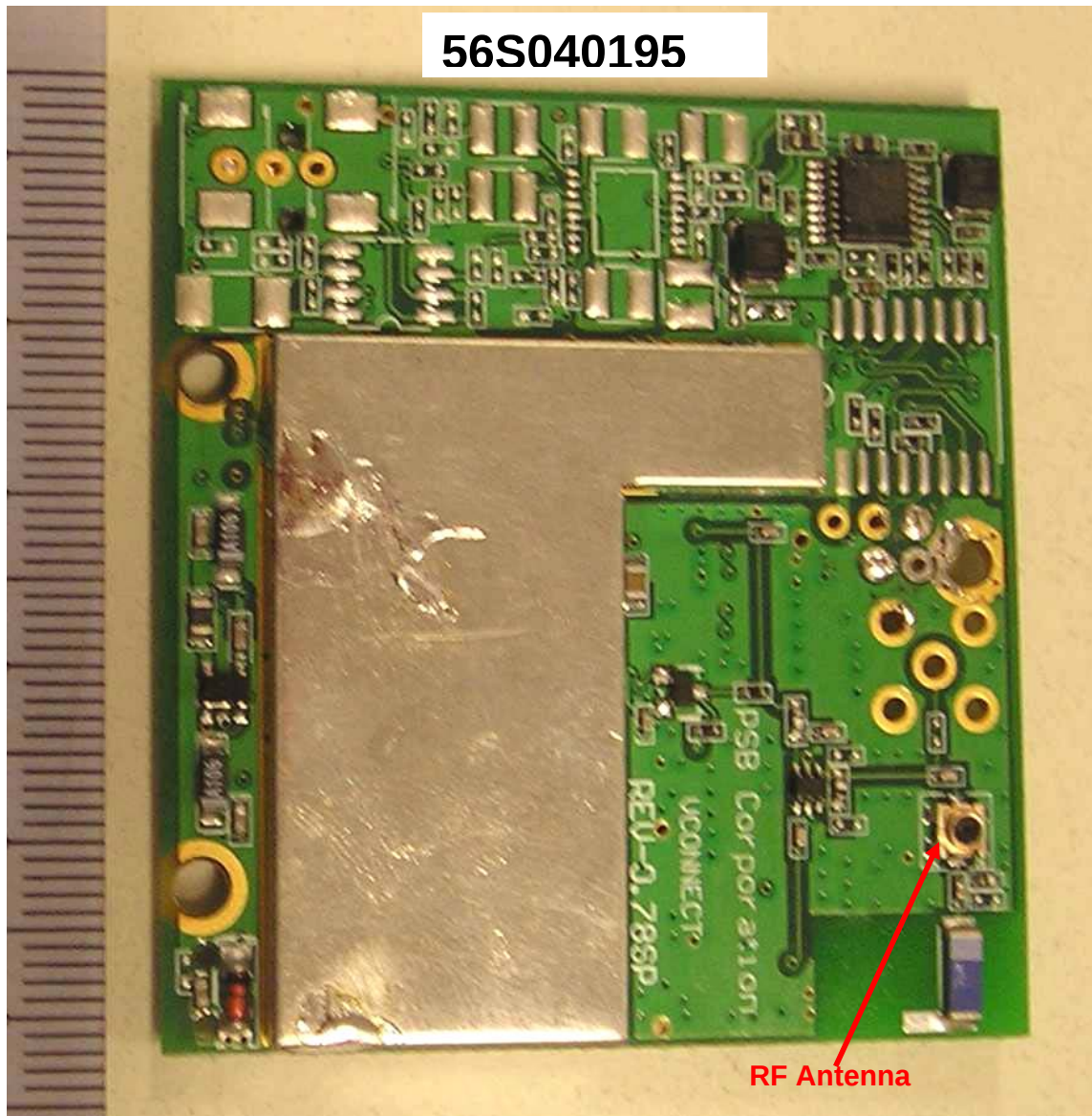
Rear Left/Right Speaker – RF Board Component Side (With RF Shield)
