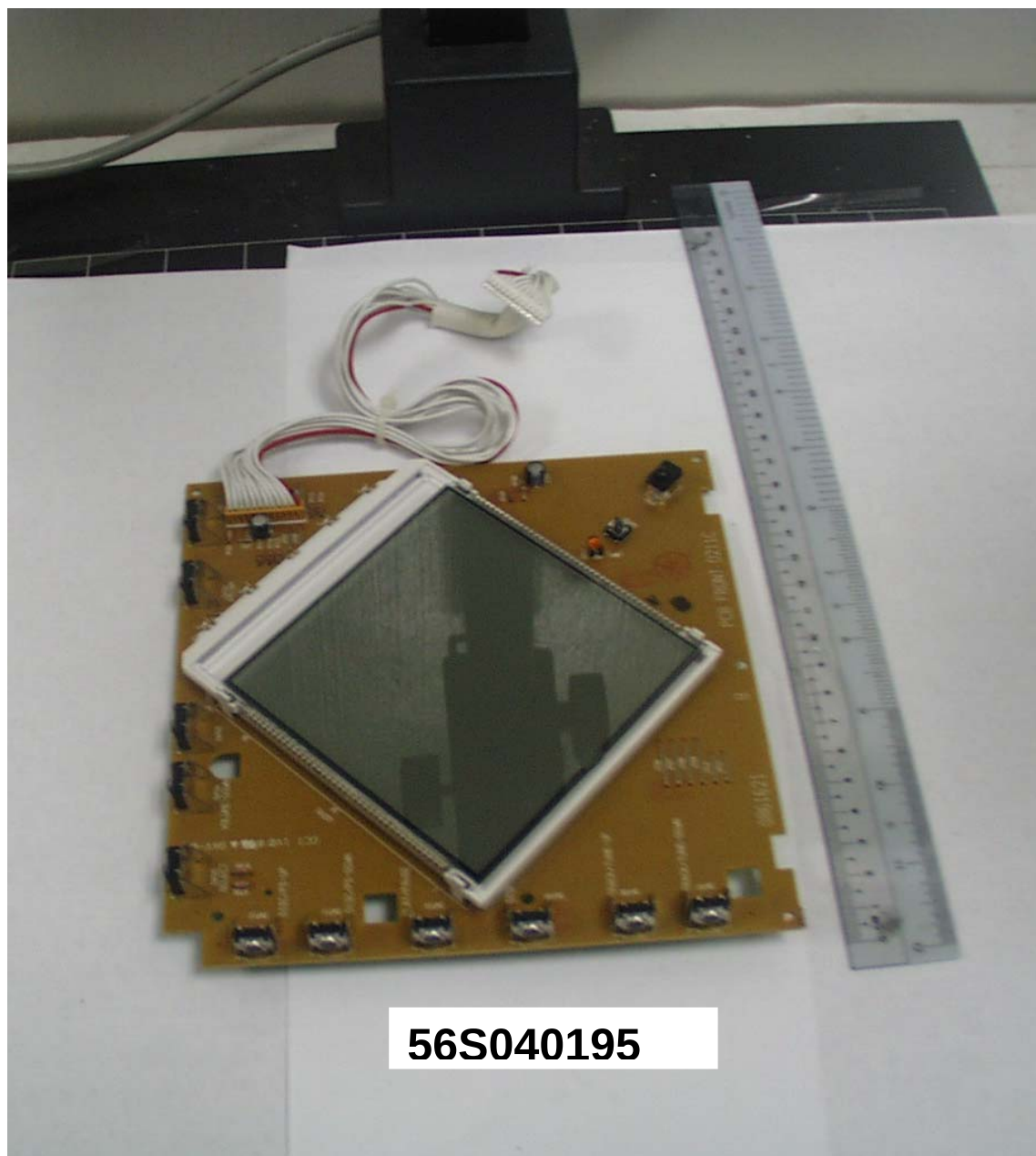
Main Unit – LCD Display Component Side
