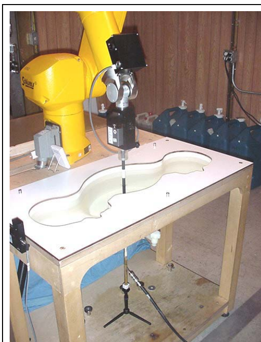
DASY4 System with SAM Twin Phantom V4.0C
