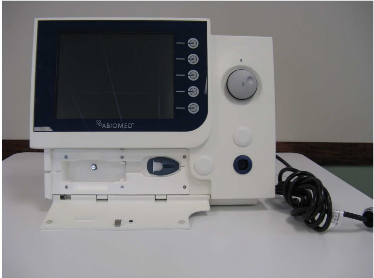
0042-4000 IMC Console – Front View – Purge Cassette Door Open
