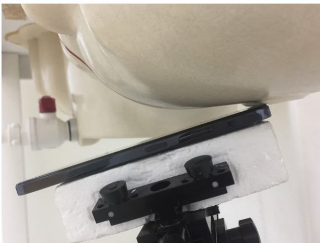
Left Tilted, Test Separation 0 mm
