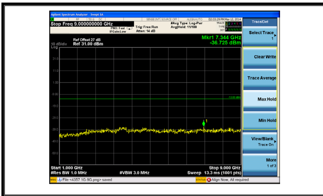
(Plot E2.1: WCDMA850MHz Channel = 4175, 1GHz to 9GHz)
