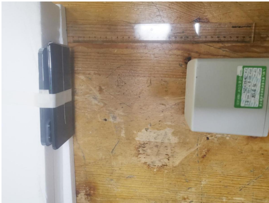
E-Field&amp;H Filed Test Setup Photo of Position Bottom (20cm)
